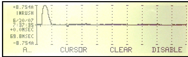
Figure 63. Amps Inrush in Normal Mode
