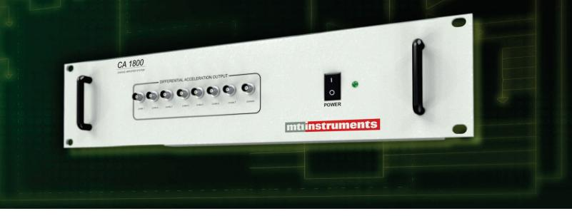
The CA1800 Charge Amplifier System conditions and amplifies charge-mode accelerometer signals. It is a rugged, rack- mountable instrument designed to be used in engine test cell control rooms and other environments where charge-mode accelerometers are used to measure machinery vibration.
