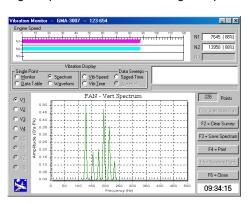
The 400 or 800 line frequency spectrum pinpoints the sources of engine vibration.
