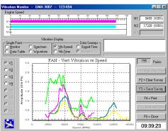
The vibration survey helps the user select the engine speeds at which balancing is required.
