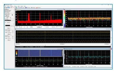
DsScopeView is a Windows based PC oscilloscope application that allows an operator to open/view and conduct playback of previous signal recordings to the display monitor for analysis, with additional display capabilities that include persistence and histogram modes.
