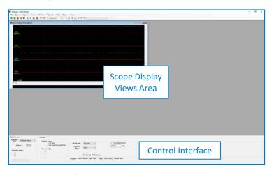
The Control Interface section provides access to the global control for acquisition and digitizer settings. A Digitizer tab is presented for each established digitizer that includes related digitizer general information panel and digitizer control panel.
