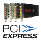
All Gage PCI Express (PCIe) CompuScope Digitizers are capable of streaming acquired waveform data through the PCIe bus directly to the host PC RAM by utilizing the eXpert PCIe Data Streaming Firmware.
