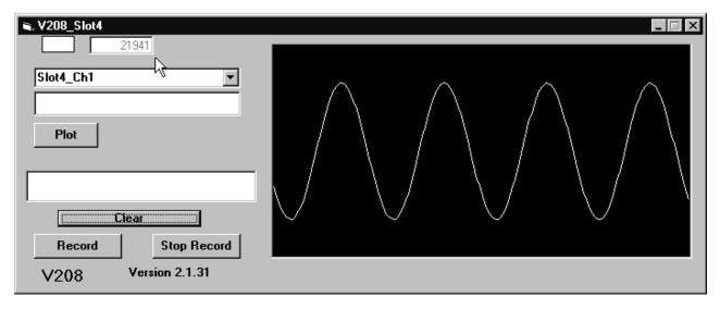
**Continuous and Transient Data Collection**—DAQ Director supports two types of data collection when used with the V200, V207 or V208 data acquisition modules from KineticSystems, continuous and transient. With other modules that do not support transient capture, such as the V213, only continuous data acquisition is provided.
