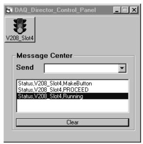
**The Data Engine**—A typical Data Engine window is shown in the figure below. Data engine windows associated with analog-to-digital converter modules contain buttons to start and stop recording to disk as well as a button to display a quick graph to check on system operation. The data engine windows are normally minimized during system operation.
