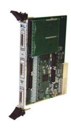
KineticSystems' CP387 is a single-width, 6U, CompactPCI module with up to 256 digital input/output channels.
