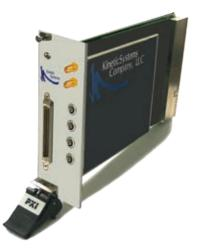
KineticSystems' P580 is a double-width 3U PXI module that functions as a multiplexer.
