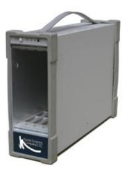
A full-size VXI mainframe with 175W Power Supply
