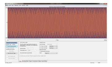
The EC14150D Scope Application software is a virtual oscilloscope application that allows the operator to view or edit all digitizer hardware settings as well as record and display acquisition data.
