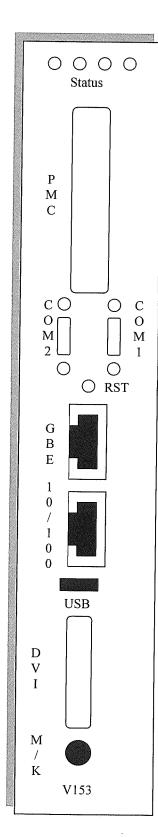
The V153 font-panel has all the standard external connections for monitor, mouse, keyboard, Ethernet, USB, and COM ports.
