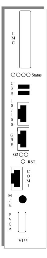
The V155 font-panel has all the standard external connections for monitor, mouse, keyboard, Ethernet, USB, and COM ports.
