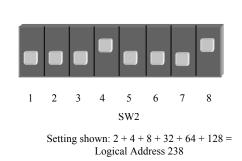
To statically assign a Logical Address to the V155, simply set the 8-position DIP switch to the desired Logical Address in the range of 0 through 254. This sets the Logical Address of the V155 and may only be altered by changing the setting on the DIP switch.
