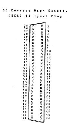
Figure 3 - 68 Socket SCSI II Mating Connector
