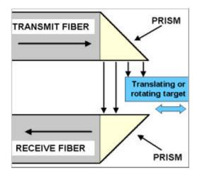
The fiber optic probe directs a "curtain" of light past the measurement target edge to an opposing receive fiber bundle. As the target moves within this "curtain", the intensity of light received changes proportionally with the edge position. The MTI-2100 Controller precisely converts this signal to an edge position or vibration amplitude.
