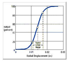
This plot shows a typical response curve for the Fotonic Edge probe that relates the amount of light received to the radial displacement of the edge under measurement. With the Fotonic Edge probe, you can make measurement as sensitive as  $0.1 \ \mu in./mV(2.5 \ nm/mV)$  over a linear range of approximately 0.004 in. (0.1 mm).
